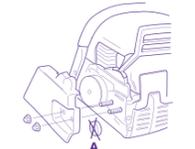
Fit the bar over the bar bolts. Place the bar in its rearmost position. Place the chain over the drive sprocket locate it in the groove on the bar. Begin on the top edge of the bar.
