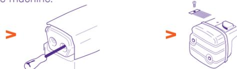
Some mufflers are equipped with a special spark arrestor screen. If your machine has this type of muffler, you should clean the screen at least once a week. This is best done with a wire brush. A blocked screen will cause the engine to overheat and may lead to serious damage.
