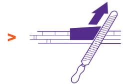
File all the teeth to the same length. When the length of the cutting teeth is reduced to 5/32 inch (4 mm) the chain is worn out and should be replaced.
