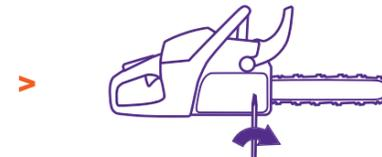
Use the combination spanner to tighten the bar nuts while lifting the tip of the bar at the same time. Check that you can pull the chain round freely by hand and that it does not sag from the underside of the bar.
