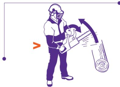
If the kickback is less violent or the kickback zone of the bar is closer to you the chain brake is designed to be activated manually by the movement of your left hand.
