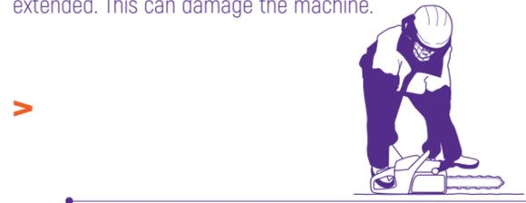
Push in the choke control as soon as the engine fires and make repeated starting attempts. Immediately press and release the throttle when the engine starts. That will disengage the throttle latch.
