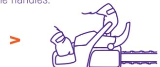
Apply full throttle and activate the chain brake by tilting your left wrist forward onto the front hand guard.
